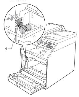
Match the guide ends (2) of the drum unit to the ▶ marks (1) on both sides of the machine, then gently slide the drum unit into the machine until it stops at the green lock lever.
